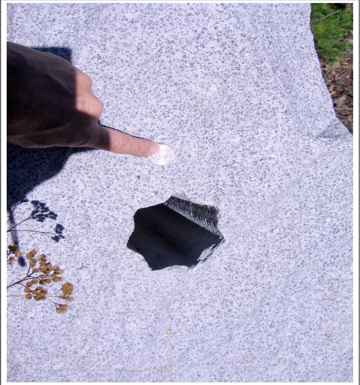
A “star” drill hole through a block of nepheline syenite at Table Mountain illustrates the ability to sharply cut the stone.
